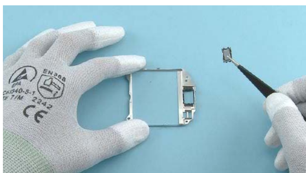
27) Remove the EARPIECE with tweezers.
