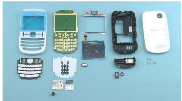
32) The Nokia Asha 200 disassembly is now complete.
